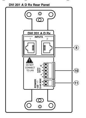
Figure 2-16 — DVI 201 Rx rear panel connectors
